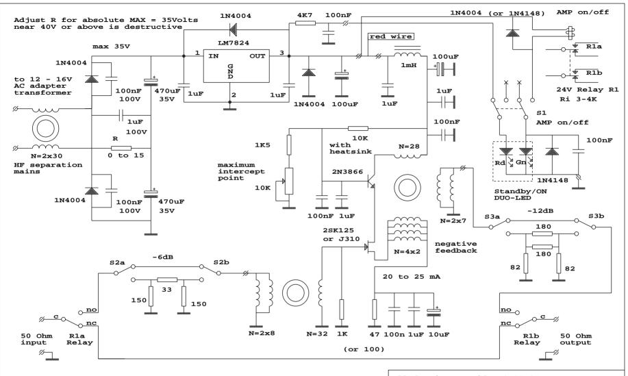
The use of a tuner with a good Q in front of the pre-amp is highly recommended. The pre-amp probably doesn't get overloaded, but your Rx will! The resistor networks are NOT to adjust the gain, but help to detect a possible cause of overload, and where!
