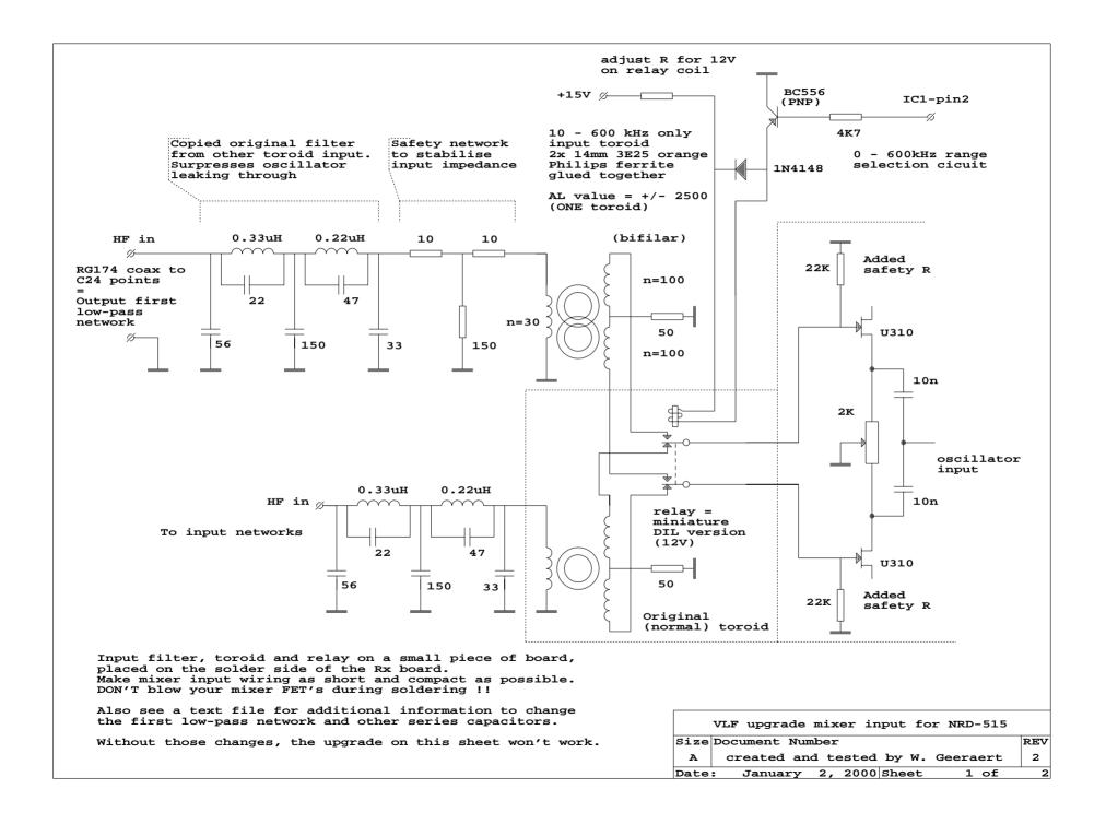
Text file belongs to the 515\_mix2 circuit. A mixer circuit change for the JRC NRD-515 receiver.
