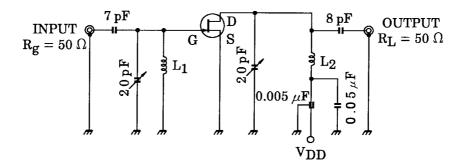
$L_{1}\!\!:0.8$  mm/  $A_{g}$  plated Cu wire 3 turns, 10 mm ID, 10 mm length
