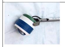
Here a coil form is used, two parts of two bottles. The coil pickup head is made rotatable. Electrical construction is the same as above. Used with a 85 mm bottle, now N = 11 Usable range from 50 Hz to 10 MHz.
