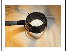
Coil form = plastic pipe. NO magnetic medium. N depends on pipe diameter, N should be equivalent to  $25 \times 25 \text{ cm}$  square. 1/16 sq. Meter. With a 70 mm pipe form (removed) N = 16.2.
