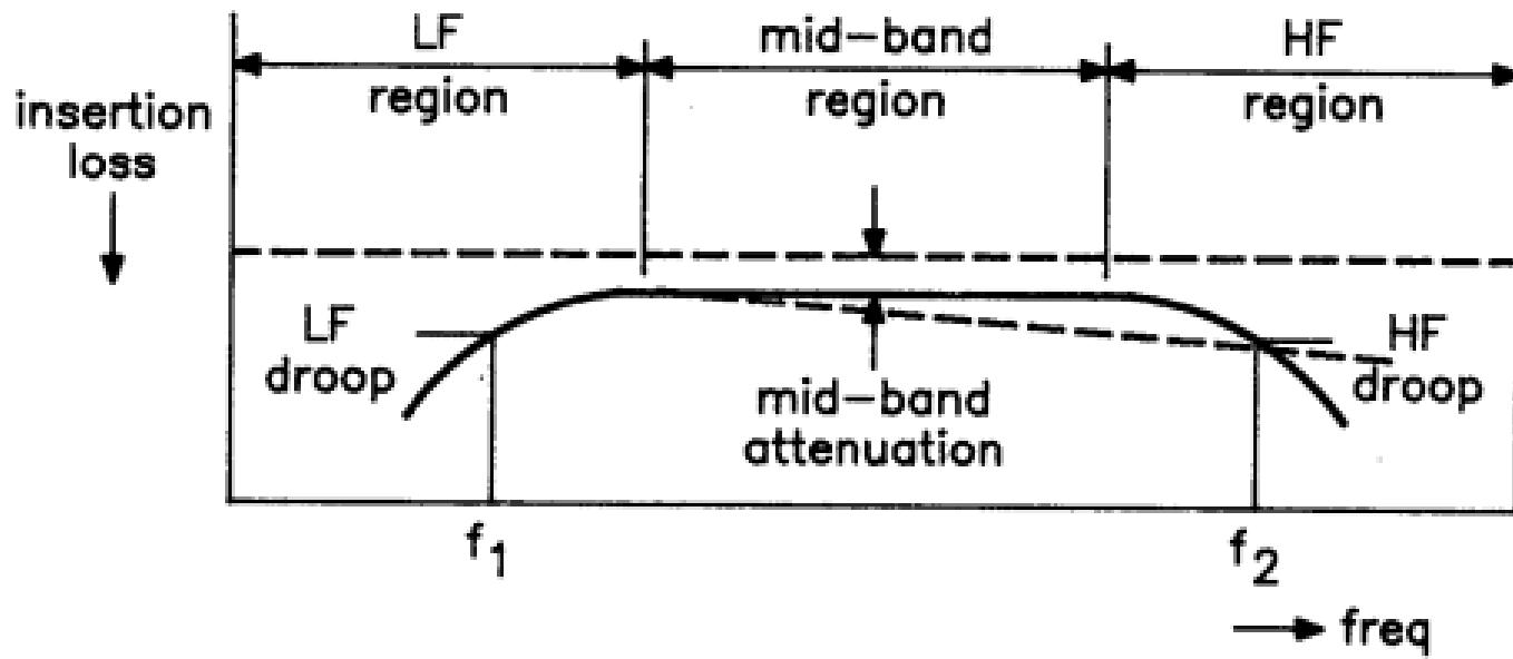
Transmission characteristic of a wideband transformer.
